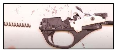
Step 18: Pull the Trigger to release the Hammer. Then locate the Small Clip on the Left side of the Assembly.
