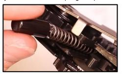
Step 24: Compress the Spring back into place with your Flathead. Then push the Tab of the Cartridge Drop Lever back over the Cap to Capture it.
