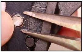
Step 28: Use your Micro-Tip to pop the Cartridge Drop Lever Spring back on top of the Small Tab.
