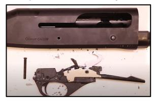
Step 31: Turn the Receiver Upright. Locate and Hold Down the Bolt Release to allow the Trigger Assembly to fit.
