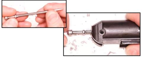
Step 15: Push in the Firing Pin so the Thin Neck lines up with the hole on the Bolt. Press the Retainer Pin back into the Bolt to Capture the Firing Pin.
