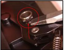
Step 26: Drop the Small Clip back over the Hinge Pin. Use your Micro-Tip to Guide it back into Place. Make sure it is Seated Tight.
