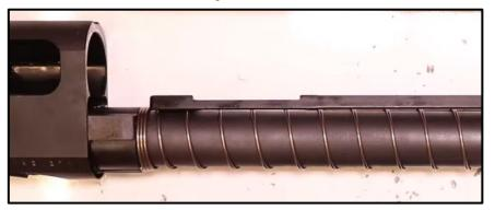
Step 35: Drop the Grooves of the Bolt into the Cutout on the Action Bar. Hold it in Place for now.
