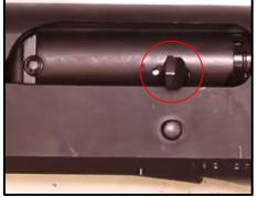
Step 39: Place the Magazine Tube Nut back on and Tighten it up.
