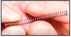
Step 14: Slide your New Firing Pin Spring onto your Firing Pin and Drop it back into your Bolt
