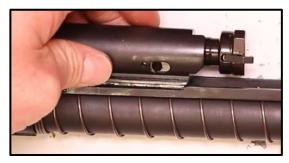
Step 36: Slide the Magazine Tube through the Forend of the Barrel.
