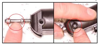
Step 16: Push on the Firing Pin. Make sure it doesn't jump out.
