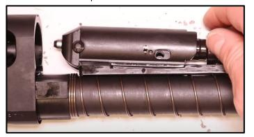
Step 7: Slide off the Action Bar and Action Bar Spring.
